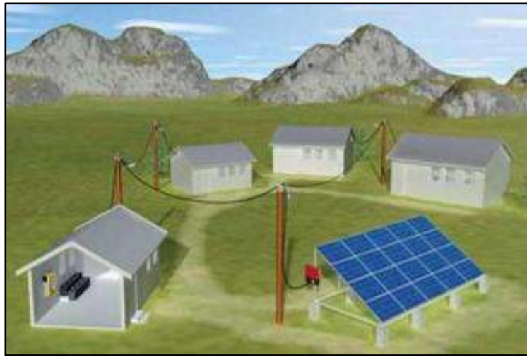
Figure 1- 2: Illustration of the components of solar mini-grids 2
