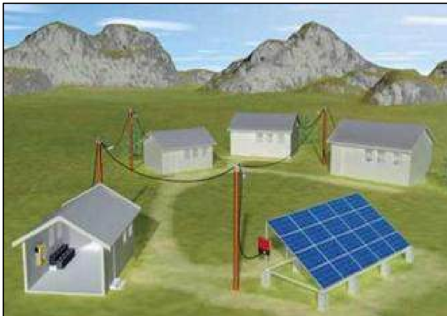
Figure 1- 2: Illustration of the components of solar mini-grids 2
