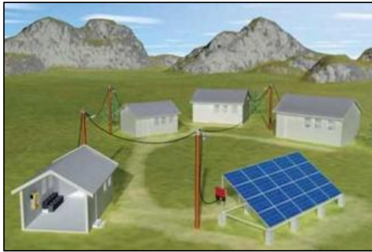
Figure 1- 2: Illustration of functions of the components of a solar mini-grid 2
