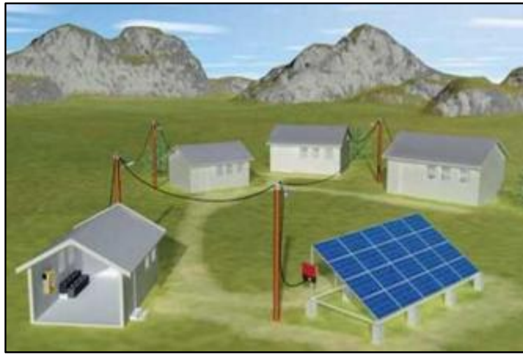
Figure 1- 2: Illustration of the components of solar min-grids 2
