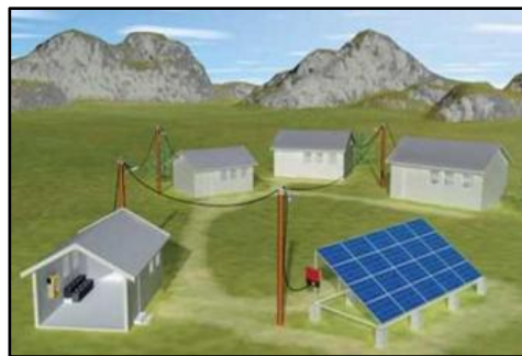
Figure 1- 2: Illustration of the components of solar mini-grids 2
