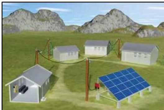
Figure 1- 2: Illustration of the components of solar mini-grids 2
